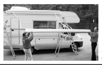
7 Slide the new canopy into the lead bar rail.
