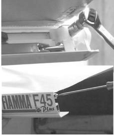
4 Loosen boltz on leg supports using a 13mm wrench and slide legs out of rail. Remove the screws which hold the canopy in the rail.
